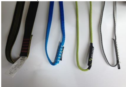
Photo 33 Different types of slings. From left; nylon, nylon/dyneema, aramid, dyneema
