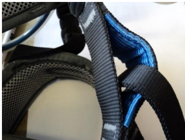
Photo 45 The wear strip on a harness
