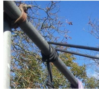
Photo 68 Three way pull on a climbing rig using an overhand, an Alpine Butterfly can also be used
